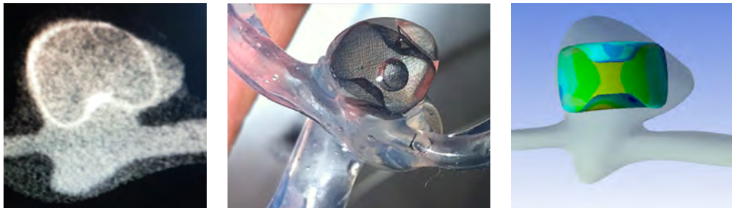
Medical devices can be tested using three methods – within the body (in vivo, left), outside the body (in vitro, center) and within a computer (in silico, right).
