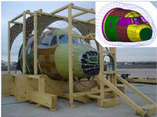
**Electromagnetic model from the digital mock-up of the cockpit**
