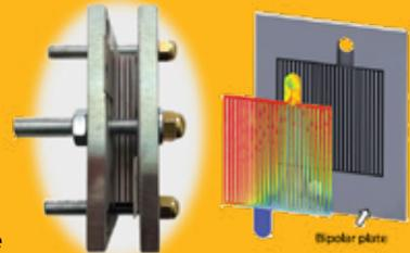
**A proton exchange membrane (PEM) water electrolysis stack for hydrogen production (left) with optimized cell design through Ansys simulation (right)**
