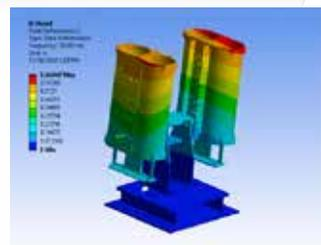
Results of the launcher shock and vibration simulation
