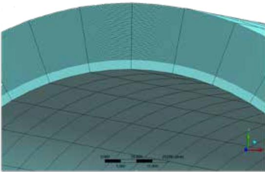
**Example of pipe body composite laminate**
