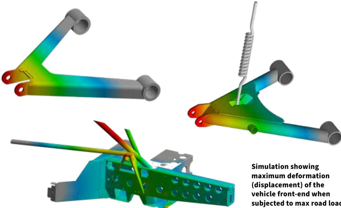
**Simulation showing maximum deformation (displacement) of the vehicle front-end when subjected to max road loads.**
