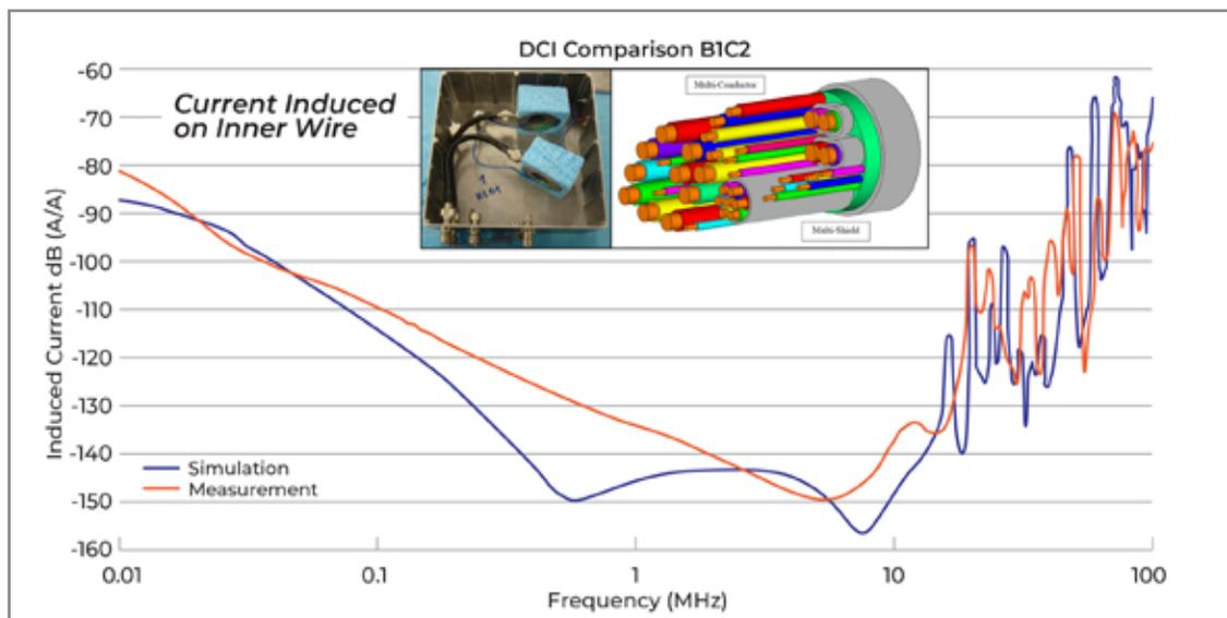
**The direct current simulation (blue) closely matched the test measurement (red).**
