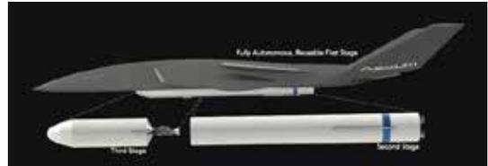
**The autonomous drone is only the first stage of a three-part system. It carries a two-stage rocket underneath it.**
