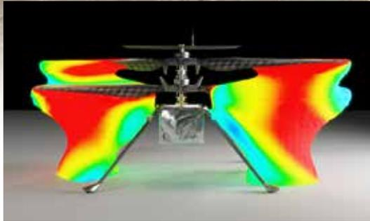
**An Ansys simulation showing zones of high pressure under the Ingenuity helicopter's rotors.**
