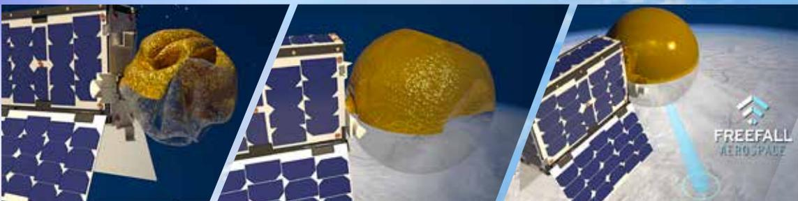
**Three of the stages of spherical antenna deployment.** Images courtesy of FreeFall Aerospace.
