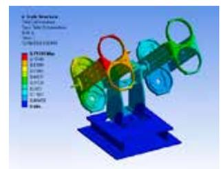
Results of the launcher static structural simulation
