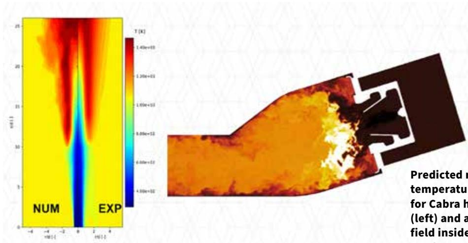
Predicted mean temperature distribution for Cabra hydrogen flame (left) and an aerothermal field inside an aero-engine combustor (right)
