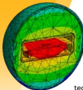
**Results of the probe thermal simulation**
