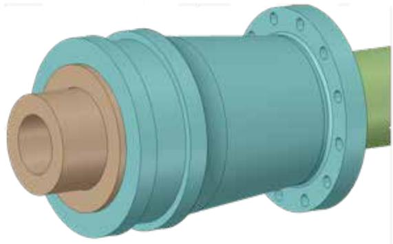
**Example of end fitting CAD geometry**
