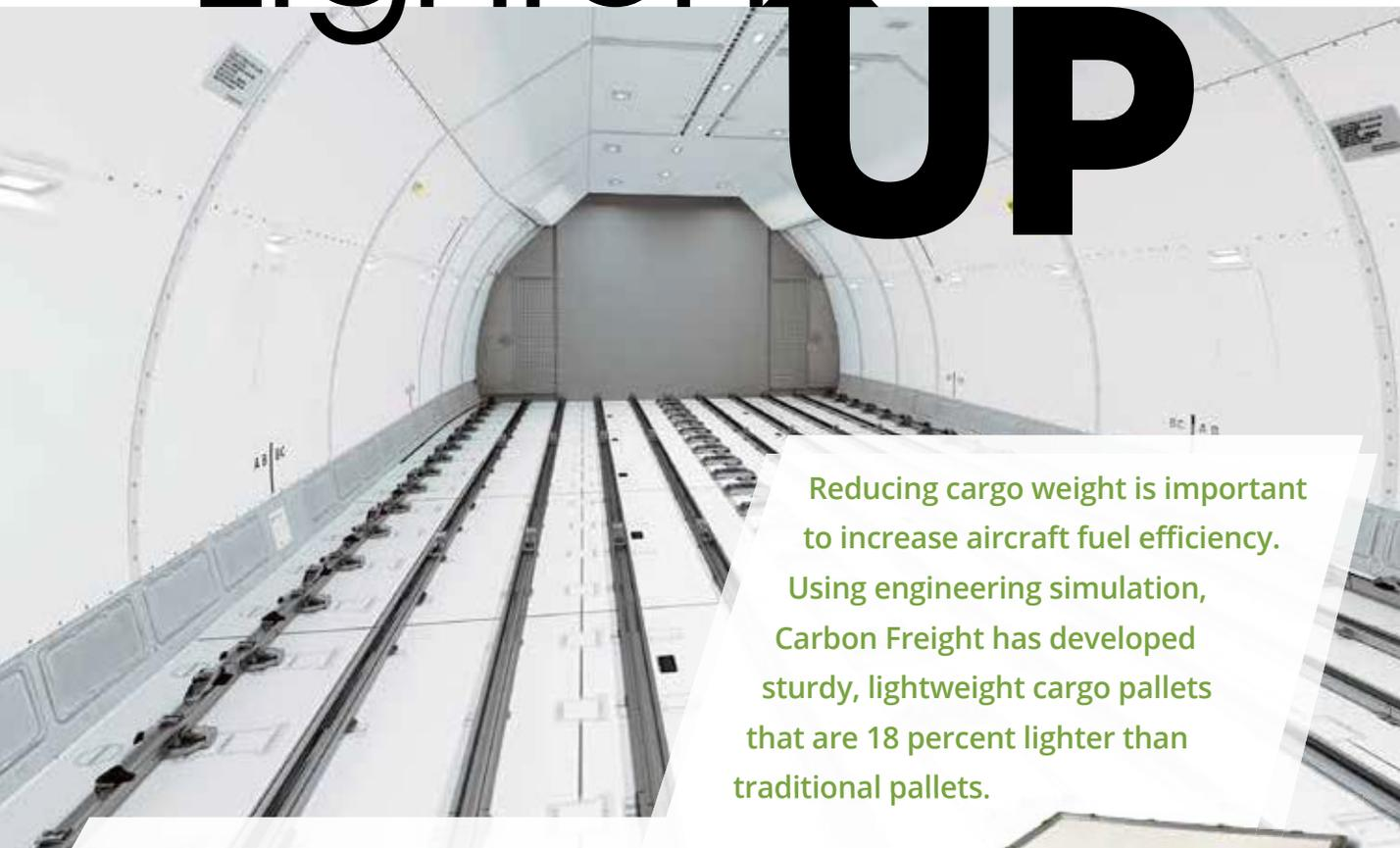
Reducing cargo weight is important to increase aircraft fuel efficiency. Using engineering simulation, Carbon Freight has developed sturdy, lightweight cargo pallets that are 18 percent lighter than traditional pallets.
