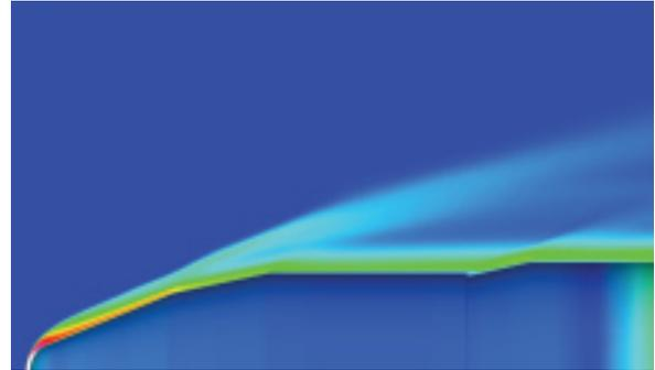
CFD contours demonstrate the heat load on the surface of the launch vehicle 152 seconds into the flight.
