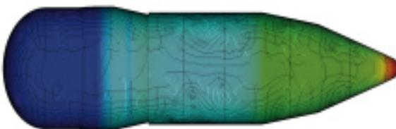
These contours represent the initial skin temperatures used for FEA simulation of the Falcon 1 launch vehicle.
