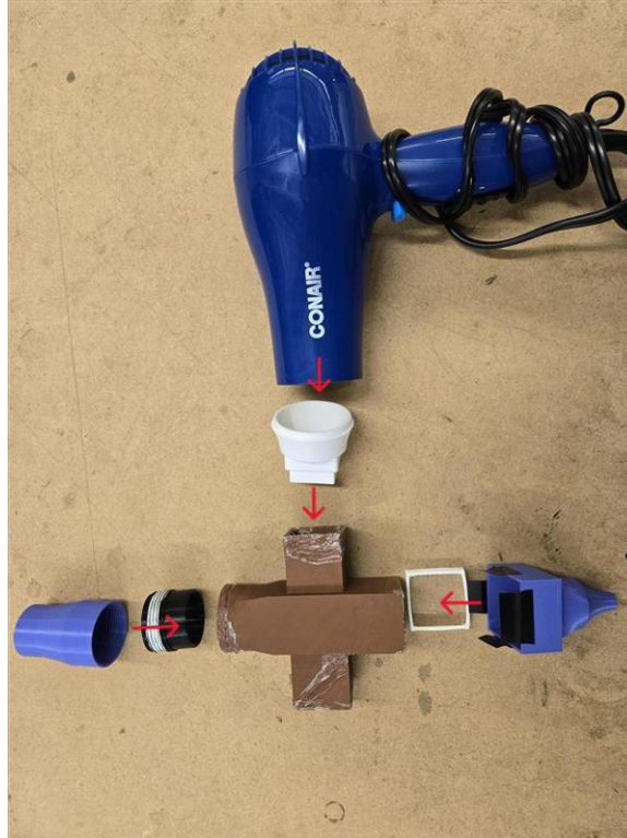
Figure 3: Heat exchanger experimental setup
