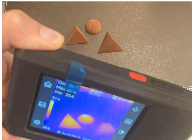
Figure 8: Measurement of the surface temperature of the 3D-printed test specimen made of copper filled HTPLA using a thermal camera.
