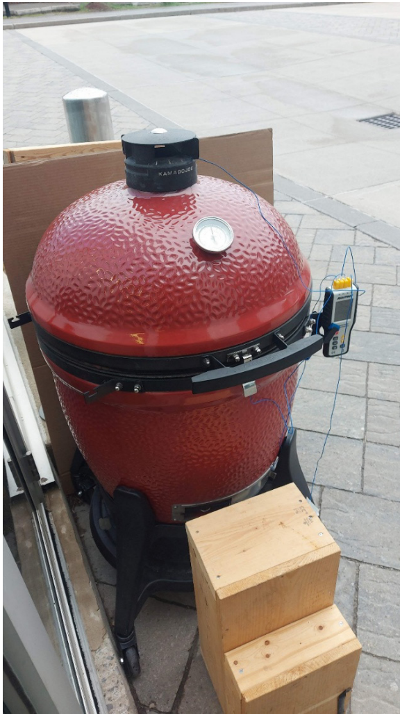
Figure 3: Experimental setup of the K-type thermocouple and the anemometer (not shown) inserted inside the barbecue (right)
