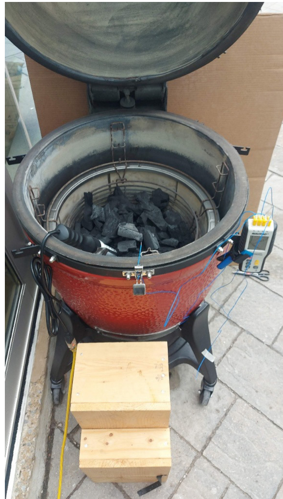
Figure 3: Experimental setup of the K-type thermocouple and the anemometer (not shown) inserted inside the barbecue (right)
