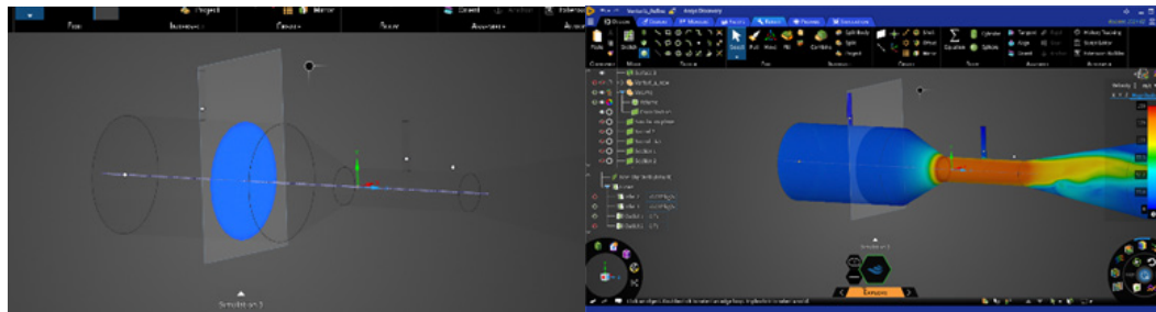
Figure 25: Converged Velocity Profile of Venturi 1. Flow direction indicated with yellow arrow
