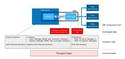
Additionally, the approved correction #167 in the FACE PR/CR Tool states that "an ARINC\_661\_Command\_Stream message type can be communicated over the TSS interface as follows:"
