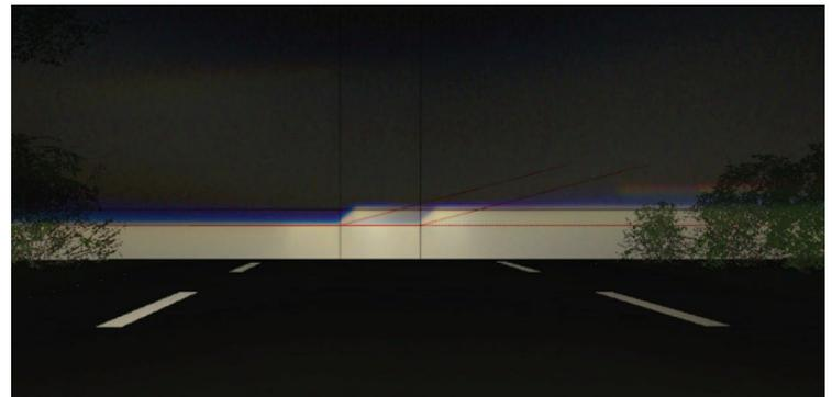
**Digital mock-Up** allows users to import vehicle shapes, used as masks, from CAD software in 3DXML to offer an assessment of the visibility when driving a specific vehicle.
