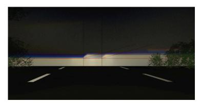
**Digital mock-Up** allows users to import vehicle shapes, used as masks, from CAD software in 3DXML to offer an assessment of the visibility when driving a specific vehicle.
