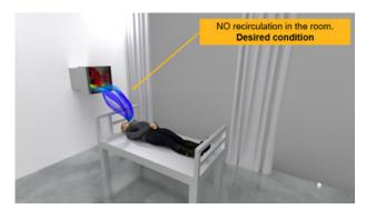
Figure 2: CFD predictions for recommended ventilation system design
