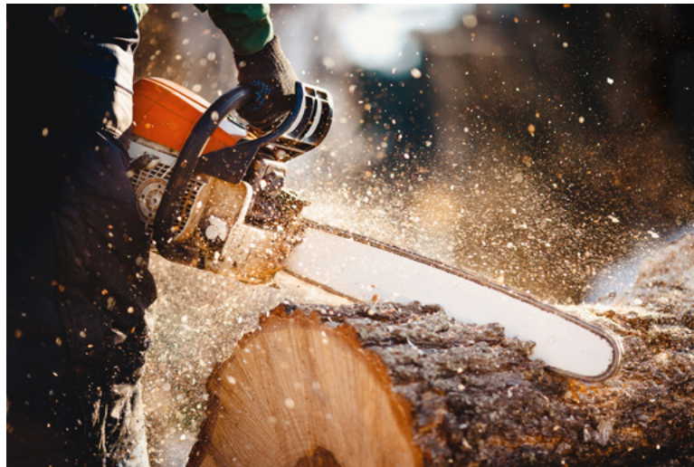
Figure 1: Close up of a chainsaw blade in action. The blade houses the chain, which does the cutting.
