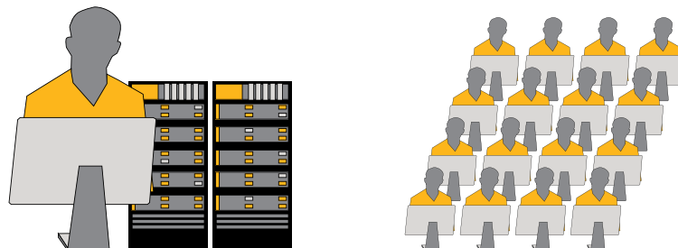
Figure 1: HPC capability and HPC capacity reflected by two different HPC usage scenarios: single user running a large job on a cluster (left image) and many users running smaller jobs on a workstation (right image).
