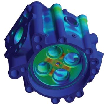
▲ Von Mises stresses caused by temperature and pressure on block
