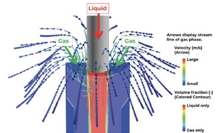
By leveraging Ansys Fluent via Fujitsu's Technical Computing Cloud, Chiyoda's engineers are able to create robust CFD models that show both flow paths and volume fractions for liquid and gas.
