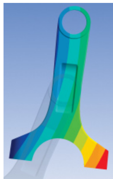
Figure 6. Results, with CMS parts, are post-processed as they normally would be in ANSYS Workbench Simulation.
