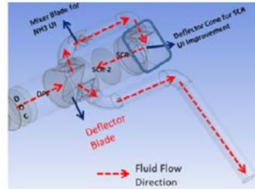
Figure 4. Pipe/cone/diffuser optimization for minimum back pressure and maximum flow distribution.
