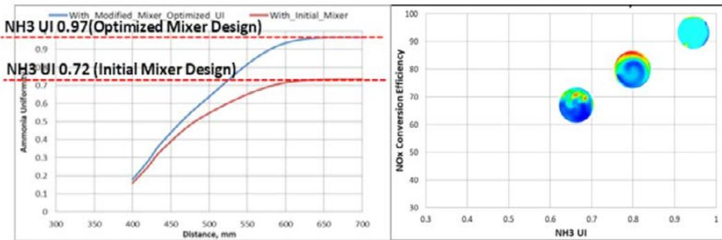
Figure 7. NH3 Uniformity Index (UI) comparison for initial and optimized design and NOx conversion efficiency with respect to NH3 UI.
