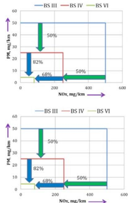
Figure 3. Emission limit for diesel (current and future).
