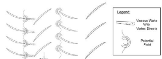
Figure 2: A depiction of the physics involved in multi-row interaction in turbomachines, showing physical wave reflection from downstream rows.
