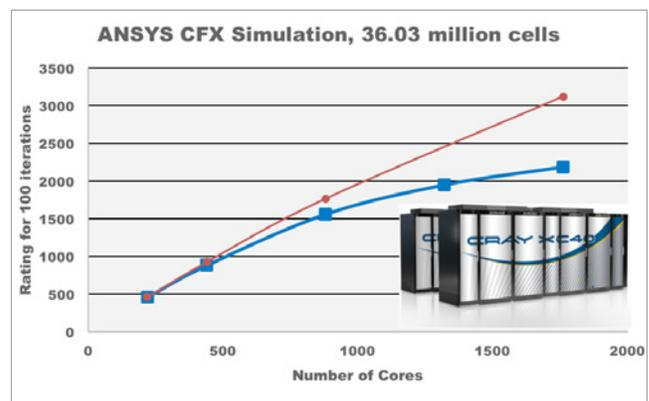
**ANSYS CFX and the Cray XC System in Action**
