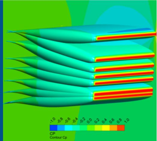
rectangular platform with a supercritical airfoil shape cross section.
