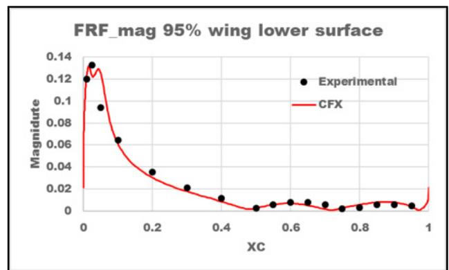
magnitude trends over the upper and lower wing surfaces are accurately captured and also match well with the experiments.
