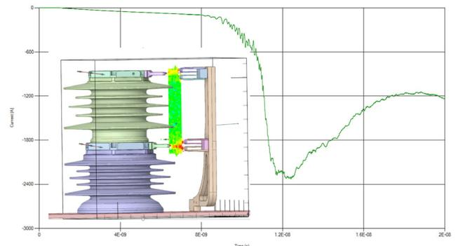
Arc Current Waveforms – EMI Testing
