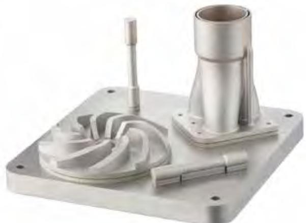
Additive manufactured parts with specimens for mechanical testing on a build plate are shown here.
