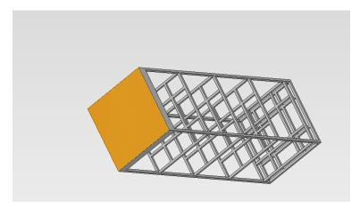
f. Finally, with the face selected go **Support 1 Panel** and in the **Location** box click the **Plus Button** to add the face to the **Support 1 Condition**.
