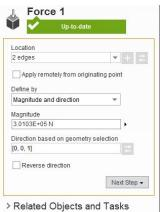
e. Click in the **Direction Based on Geometry Selection** section and **select an edge that is perpendicular** to the edges you selected for the **Location**
