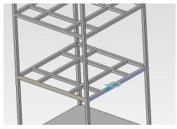
f. Back in the **Force 1** menu click on the **Replace** button in the **Direction Based on Geometry Selection which** which will change the direction of the arrow to facing directly at the beam selected earlier.
