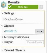
d. Now we can see the results by click on the word <u>Results</u> in this panel. Doing this will bring up another panel with two items, <u>Equivalent Stress</u> and <u>Displacement Magnitude</u>. <u>Clicking the arrows located in the top-left</u> will allow you to navigate between the two results.
