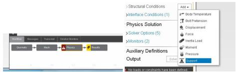
b. The **Support 1 Panel** will open in the top left of the screen and under the **Location** box we will need to add the area of our model where the support of the ground will be located. In our case it will be at the bottom of our **Foundation**.
