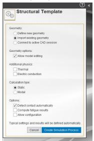
d. Click <u>Create Simulation Process</u> and a window will open to <u>Import Existing</u> Geometry, which is where you will select your <u>STEP File (.STP)</u>
