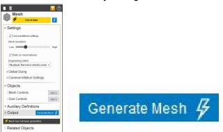
c. The building will now look like it has a net all over it which is the **Mesh.** The mesh represents the discretization of the physical domain into a mathematical model. The mesh enables AIM to assemble a system of equations, which are used to compute the physical response of the domain.
