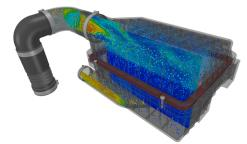
Discovery accounts for porous media to evaluate porous materials such as filters, screens and perforated plates within a product design.
