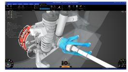
Explore multiple manufacturable designs in minutes through a fast and interactive experience, where you can define objectives easily and apply controls to ensure that manufacturing requirements are met, minimum material thicknesses are set and exclusion areas are defined.
