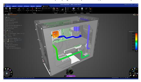
Leverage conjugate heat transfer (CHT) to determine fluid and solid temperatures for evaluating fluid and thermal performance of product designs.
