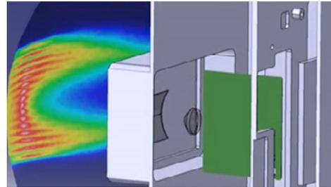
Ansys SPEOS enables engineers to simulate the optical images that are gathered by cameras and lidar systems mounted on the VTOL vehicle — critical in ensuring that the craft can accurately sense and respond to its physical surroundings.
