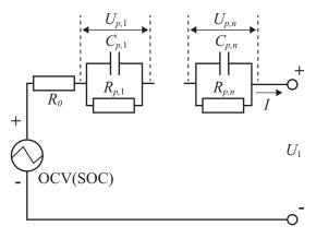
The 2RC model representing the Li-ion battery cells' temporal thermal and electrical performance
