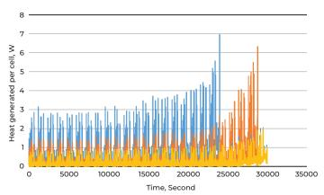
shock can pierce or puncture them, and This graph shows the typical heat-generation data from an equivalent circuit model of Li-ion cells. Color indicates the impact of operating temperature on the rate of heat generation.
