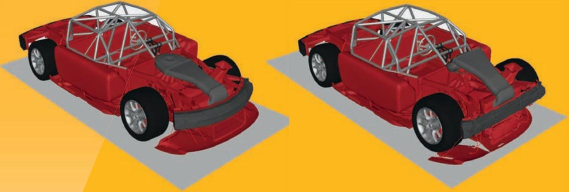
**After more than 5,000 Ansys LS-DYNA crash test simulations, it took only two physical crash tests to verify and validate that the design was safe.**
