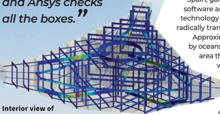
**Interior view of the tension leg platform (TLP) floater, to which the mooring lines are connected**
