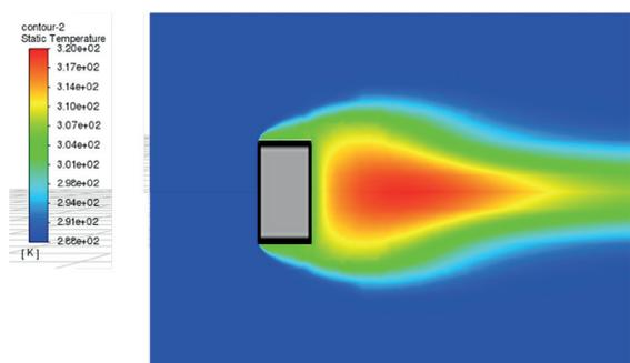
**Figure 6: Temperature contours across a horizontal plane of constant height 1.8 meters. In this model, the wind at 20 meters per second is coming from the left side of the graphic.**
