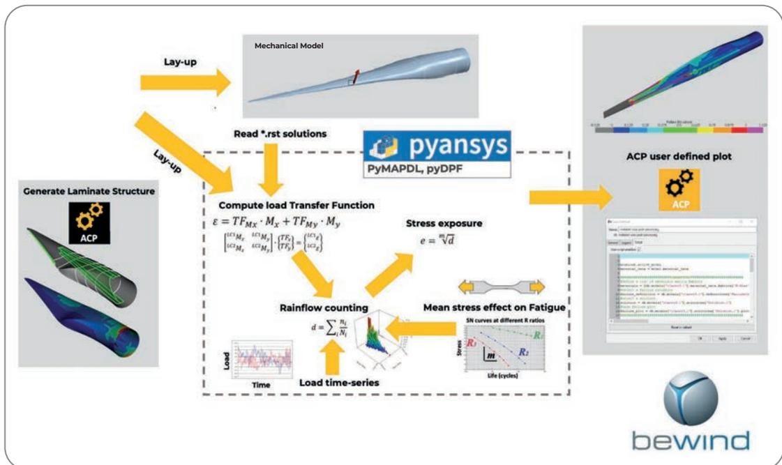
**Figure 1. Illustration of Bewind’s integration of PyAnsys with two templated load cases to compute load transfer functions at varying stress levels at each composite layer using the binary result files of a rotor blade model.**
