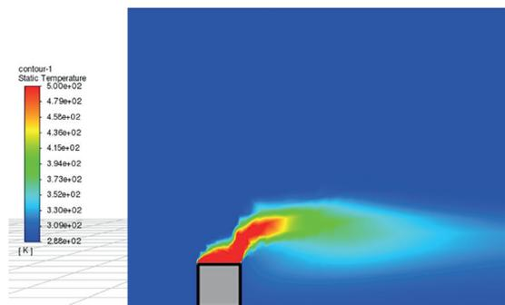
**Figure 5: Temperature contours across the central plane of the model (through the hydrogen release point) for a 3D model with incident wind speed of 20 m/s from the left**
