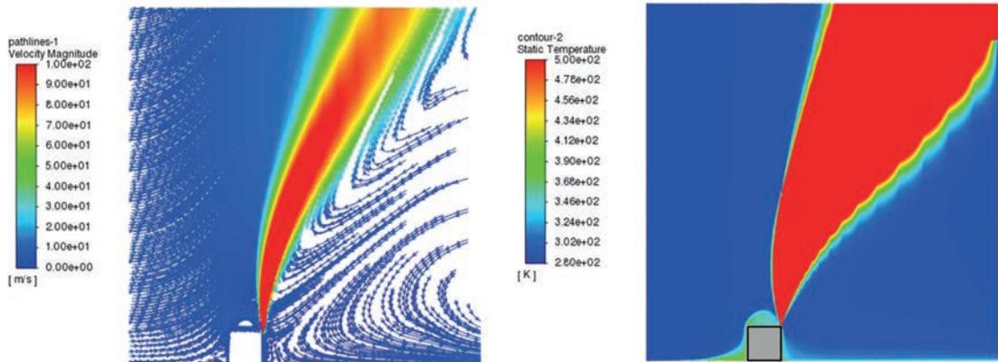
**Figure 4: Velocity colored streamlines and temperature contours for a 2D planar thermal pressure release device (TPRD) model with 5 m/s wind coming from the left**
