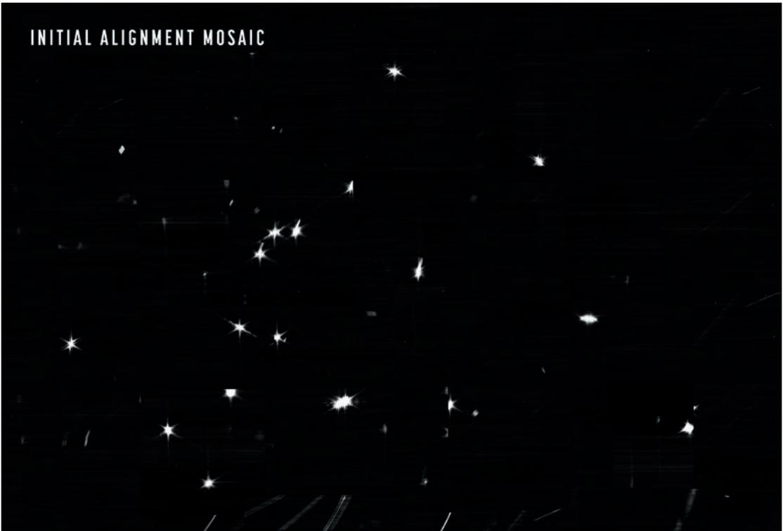
**The JWST's first blurry image of a single star, appearing 18 times for each of the 18 unaligned mirrors. When the mirrors are aligned, the star will appear as a single sharp image.**
