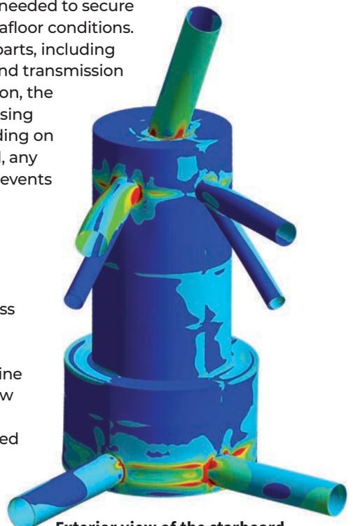
**Exterior view of the starboard main column with the pontoon termination in an extreme load case**
