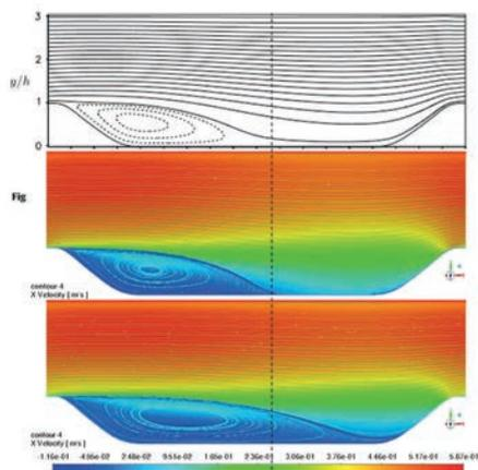
**Turbulence modeling using large-eddy simulations and Reynolds-averaged Navier-Stokes (RANS) equations, with generalized k-omega (GEKO) models.**
