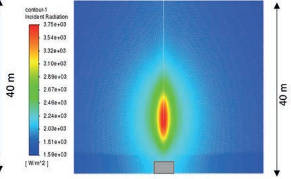
**Figure 3: Radiation profile illustrates the thermal release of nine cylinders.**
