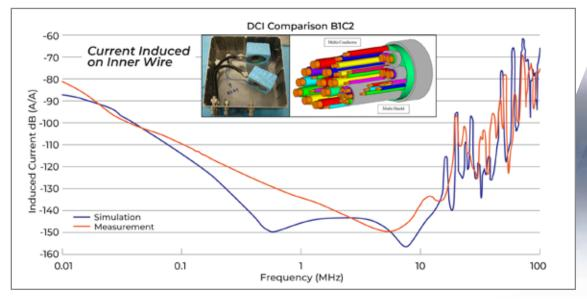
The direct current simulation (blue) closely matched the test measurement (red).
