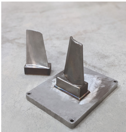
Figure 6. Comparison between turbine blade printed on the base and after removing and machining.
