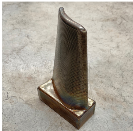
Figure 7. Turbine blade printed (DED) removed from the base.
