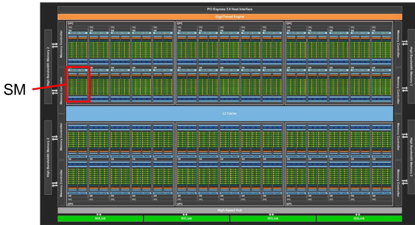
Tesla P100 Layout: 56 SMs, 3584 CUDA cores
