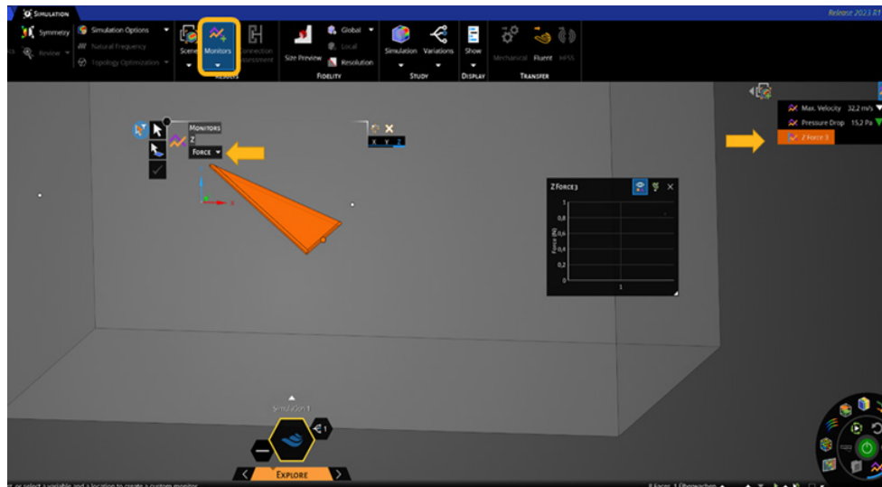
Figure 8: Drag and lift monitor applied via box-select to the internal surfaces of the fluid domain which represent the delta wing geometry.
