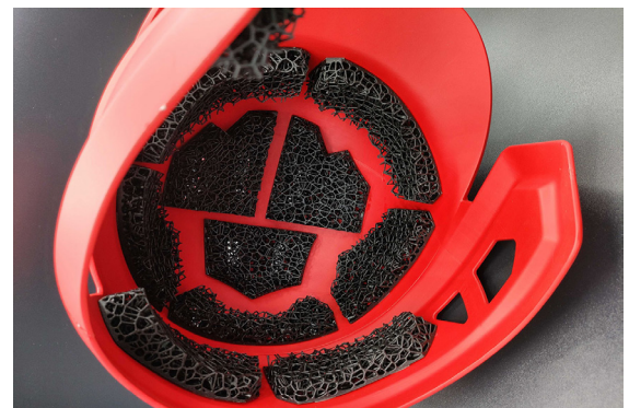
3DPC uses Ansys' simulation tools during additive manufacturing to enhance part quality, such as the 3D printed cushioning in this helmet
