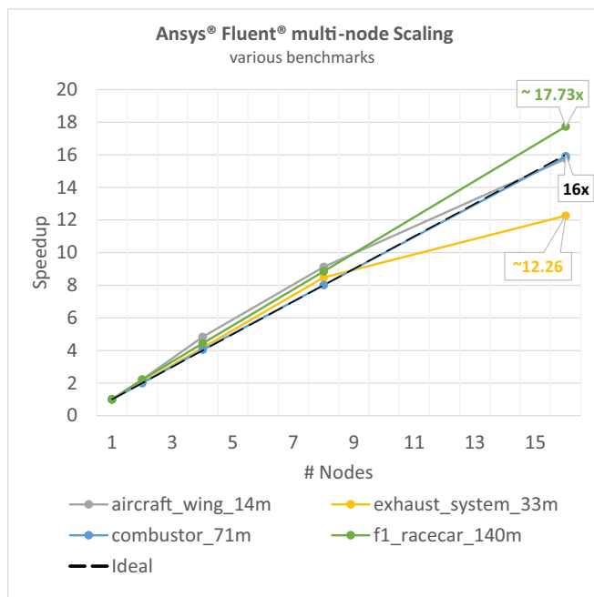
Figure 1: Ansys Fluent multi-node scaling on a variety of Ansys benchmarks.
