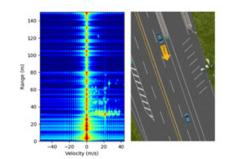
The parametric model considered radar layout (Rx and Tx positioning, number of channels, interleave mode, etc.) to fit to specific automotive radars device including Multiple Input Multiple Output (MIMO) and multi-mode (SRR, MRR,
