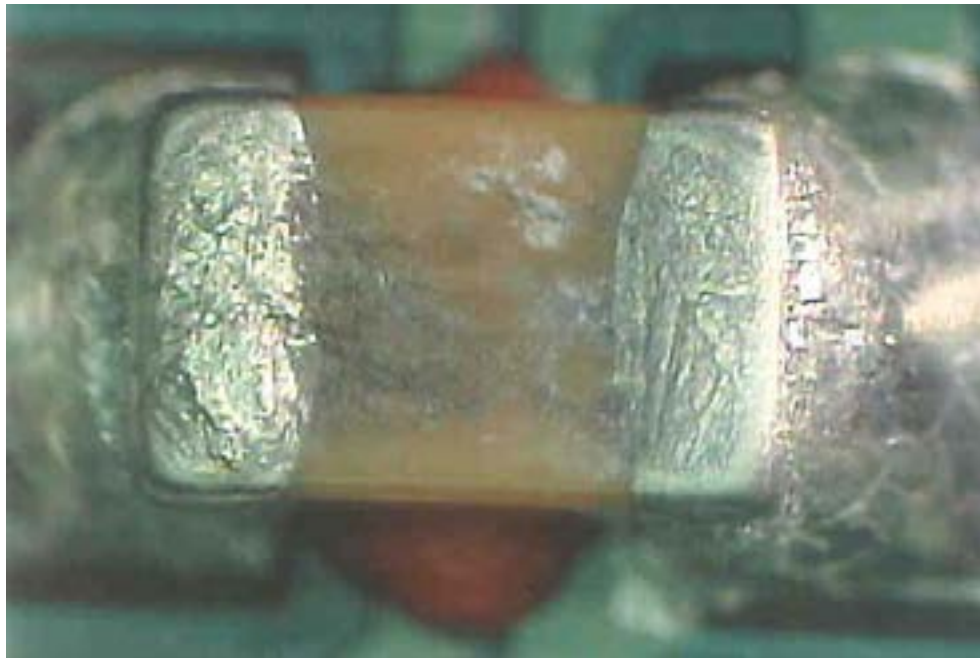
Figure 14: Optical micrograph of dendritic growth on the surface of an MLCC
