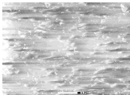
Figure 3. SEM cross-sectional view showing an enlarged image of the inner core of the CEM substrate (320x)
