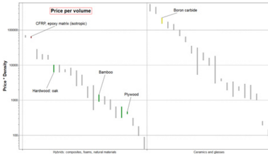
Chart: Boron carbide (and CFRP) usually have very good performance but are also very expensive. Wood costs less.
