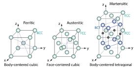
*Ferritic* stainless steels rely on *added Cr* and contain small amounts of C, usually less than 0.10%. These are the cheapest and are popular in, e.g., cutlery. Mo can be added for aggressive conditions such as sea water. Ferritic steels are ductile but not as formable as Austenitic stainless steels.
