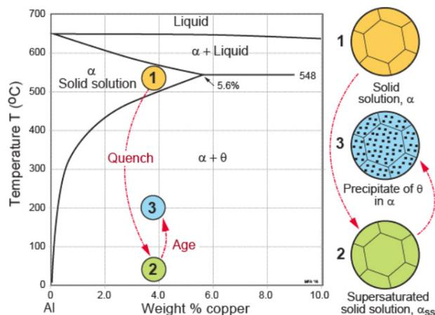
In the diagram above, an Al alloy with around 4 wt% copper is solution heat treated at 550 °C, allowing the Cu to complete dissolve into solid solution (Step 1). Upon cooling/quenching to precipitate
