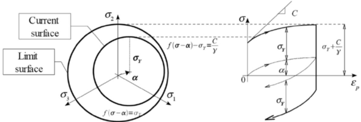
Figure 7. Nonlinear kinematic hardening using the Armstrong-Fredrick law
