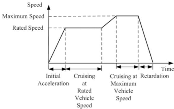
Figure 3. Representative duty cycle of an IC engine
