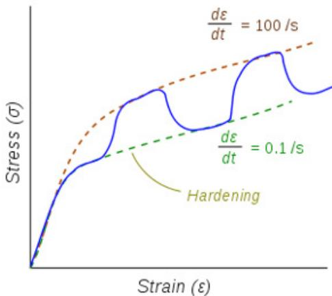
Figure 9. Viscoplastic effects as one moves between two strain rates
