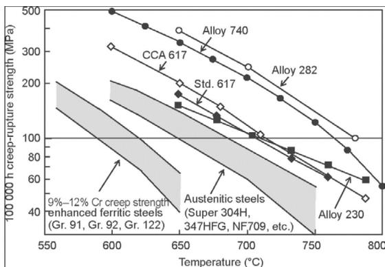
100,000-hour creep-rupture strength of some Ni-based super alloys, together with ferritic steels and austenitic steels, as a function of temperature (Abe, 2015)
