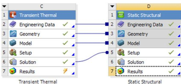
Figure 12. ANSYS WorkBench schematic for solving for thermo-mechanical fatigue
