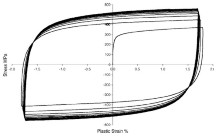
Figure 6. Typical isotropic hardening behavior seen with cycling
