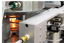
TMF test of round specimen, using induction heating, active air cooling and high-temperature extensometer
