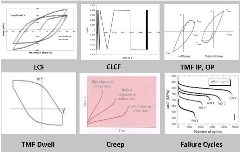
Physical testing typically takes a few months and results in 100+ tests in which the sample is tested to failure. This testing also helps in understanding the lifing characteristics of the material under different conditions.
