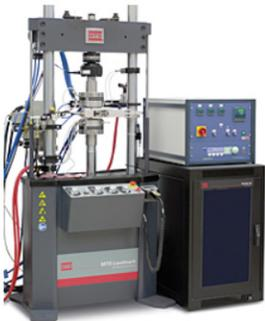
MTS Landmark® test system configured for thermomechanical fatigue (TMF) testing
