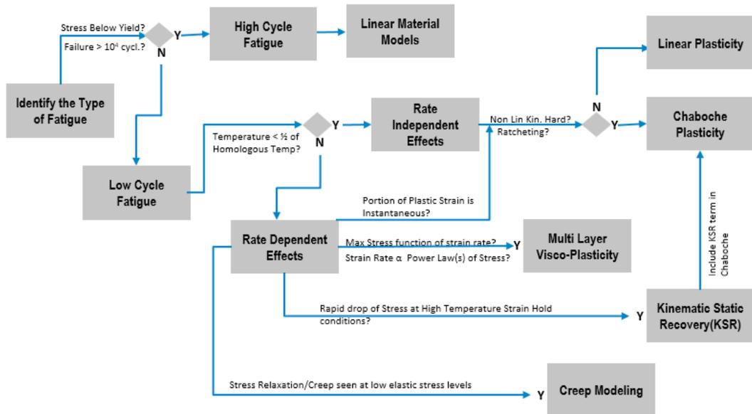
Figure 11. Material model combination decision-making tree for fatigue
