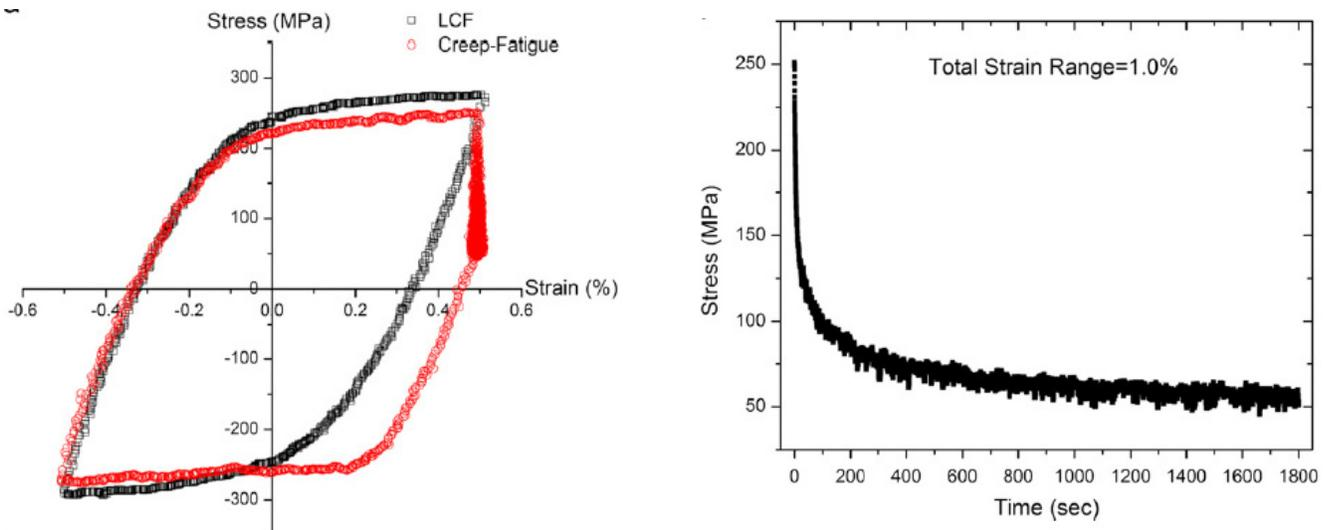
Figure 10. Stress drop in Ni-based alloy 230 at 850 C (Chen et al.)
