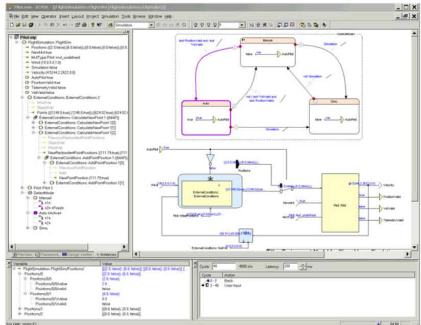
Figure 10: SCADE Suite simulation of a software module.
