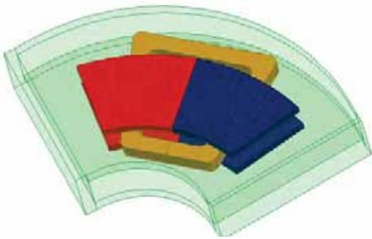
Figure 1. Voice coil motor geometry in HDD application. Blue and red segments are permanent magnets; green structure is magnet keeper, which completes magnet assembly. The voice coil (orange) moves in a rotary fashion in the air gap between magnets.
