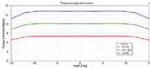
Figure 4. Torque exerted on coil as function of coil angular position for various currents applied to coil
