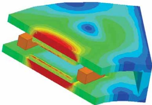
Figure 2. Magnetic flux density magnitude distribution on magnet assembly of HDD voice coil motor model in ANSYS Maxwell
