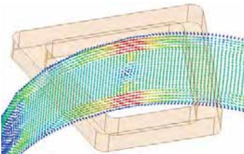
Figure 3. Flux density vector plot on curved surface in center of magnet assembly of HDD voice coil motor model in ANSYS Maxwell
