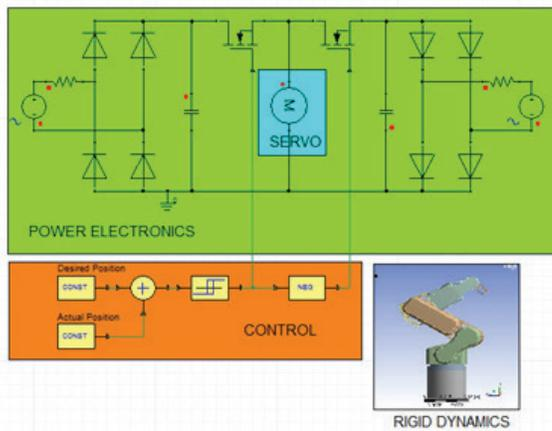
Figure 2. ANSYS Simplorer schematic shows power electronics, servo and control subsystem models together with the rigid dynamics. This represents the 3-D robotic arm system assembly.
