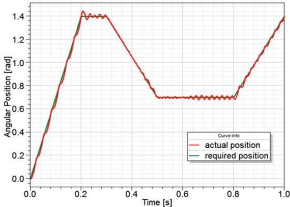
Figure 3. Actual rotational position compared to required position for one robotic arm, determined by ANSYS Simplorer model that employs cosimulation with ANSYS Rigid Dynamics
