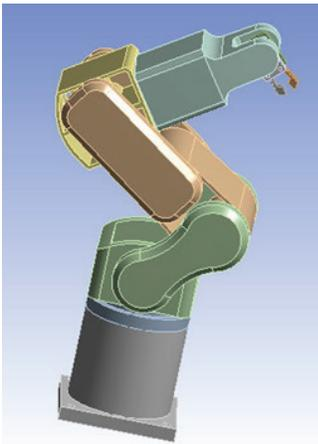
Figure 1. Robotic arm system with five revolute joints
