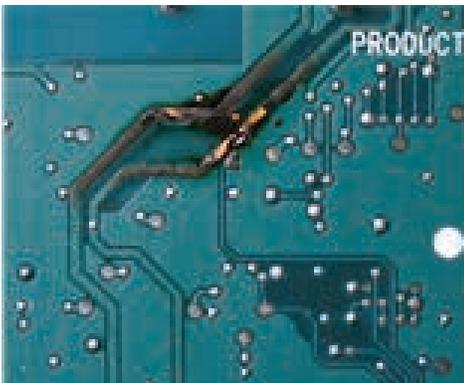
Figure 1. Fused electronic trace due to current overload. A multiphysics simulation can evaluate the combined electrical and thermal effects that lead to this failure.
