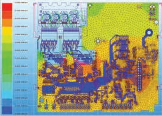
Figure 3. DC solution from SIwave. The solution provides current density, which can be used to determine areas of high current density where board or via damage may occur as a result of current overload.
