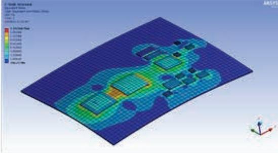
Figure 5. Thermal–stress solution using ANSYS Mechanical. Stress results consider the thermal gradients and coefficient of thermal expansion mismatch between the printed circuit board and components.
