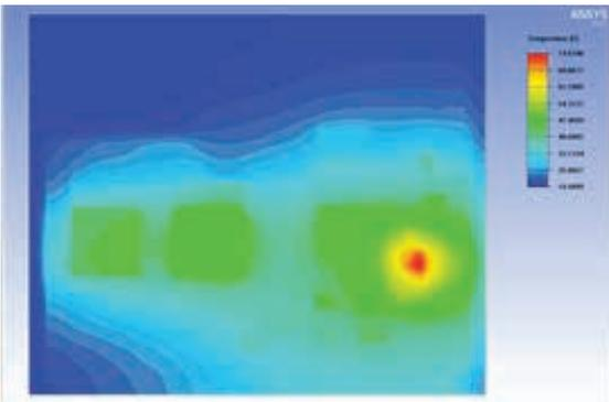
Figure 4. Thermal solution from ANSYS Icepak. Temperature results indicate a hot spot on the board that is caused by power dissipation in the metal trace layers. This hot spot could not be detected without a multiphysics simulation.
