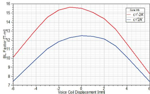
Figure 3. BL-factor, also called force factor, as a function of voice coil displacement for coil current of same magnitude but opposite polarities
