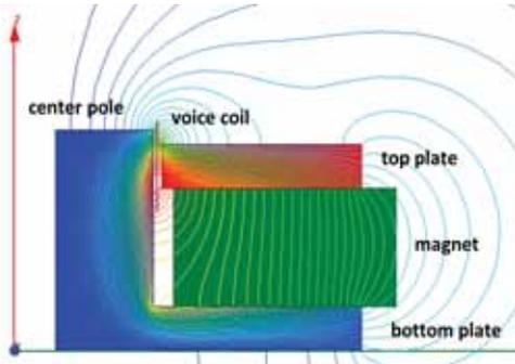
Figure 1. Typical axisymmetrical geometry of moving-coil loudspeaker magnet assembly together with flux lines plot
