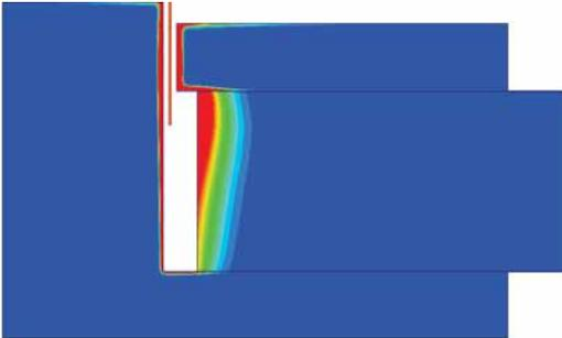
Figure 4. Distribution of power loss density in magnet assembly of modeled loudspeaker as obtained from transient simulation at 500 Hz frequency using ANSYS Maxwell
