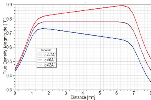
Figure 2. Flux density magnitude along line in center of air gap as a function of various coil currents
