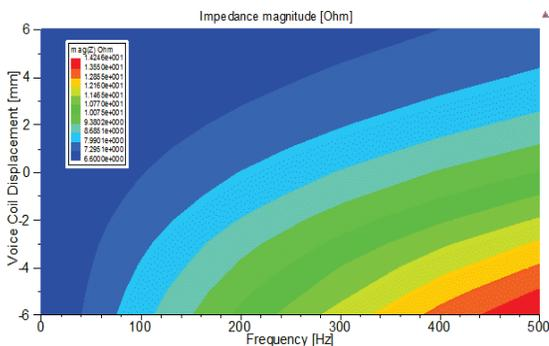
Figure 5. Stationary impedance magnitude as function of frequency and displacement of coil as obtained from transient simulations using ANSYS Maxwell
