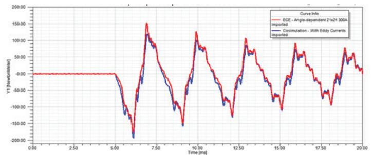
Figure 6. Comparison of short-circuit air-gap torque: ECE vs. transient FEM cosimulation
