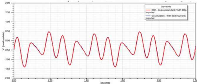
Figure 7. Comparison of cogging torque at no-load: ECE vs. transient FEM cosimulation
