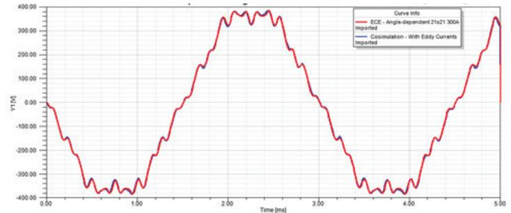
Figure 8. Comparison of back-emf at no-load: ECE vs. transient FEM cosimulation
