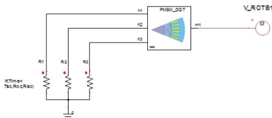
Figure 3. Simplorer test circuit: constant mechanical speed of 5,000 rpm, resistive load on stator windings switched from 1,000  $\Omega$  to 0.1  $\Omega$  at  $t = 5$  ms
