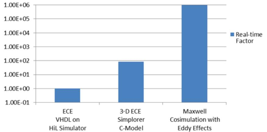
Figure 4. Real-time factor (ratio of simulation time to real-time) for various ECE and cosimulation models
