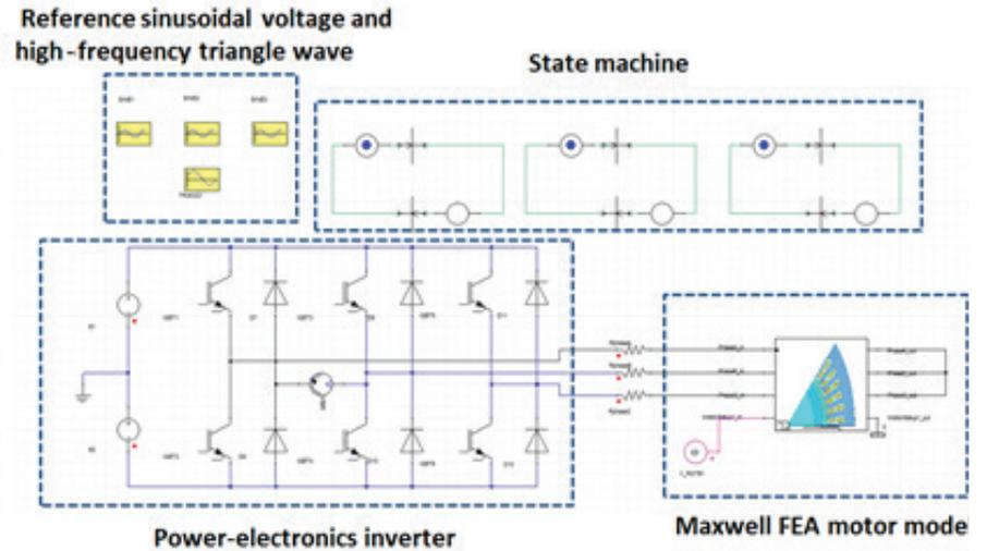
Figure 1. AC motor drive system in Simplorer using control blocks for reference voltage and high-frequency triangular waveform, state machine for control logic, power electronics inverter using system-level IGBTs, and finite element Maxwell motor model
