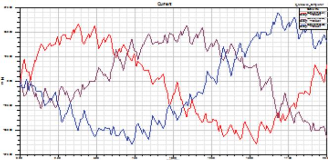
Figure 4. Three-phase current waveforms generated by inverter to drive Maxwell motor model
