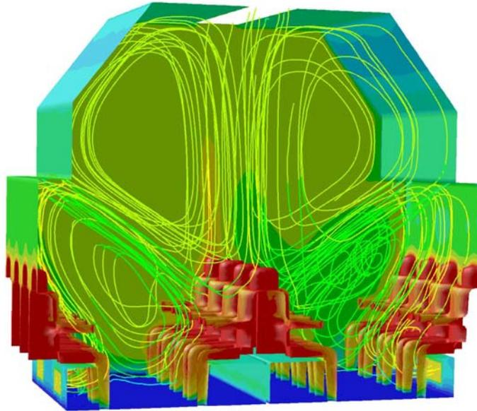
*Fig. 1:* Path lines within the cargo hold of the A400M occupied by passengers.
