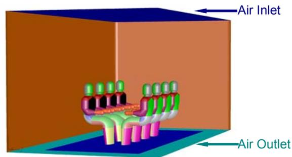
Fig. 4. Computational set up of Fanger experiments.
