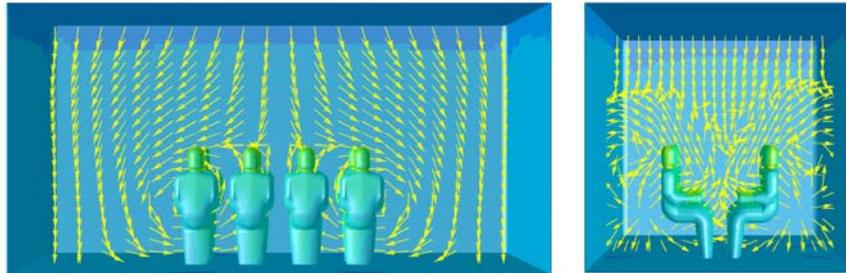
*Fig. 5:* Airflow velocity vectors in midplanes of VCC.
