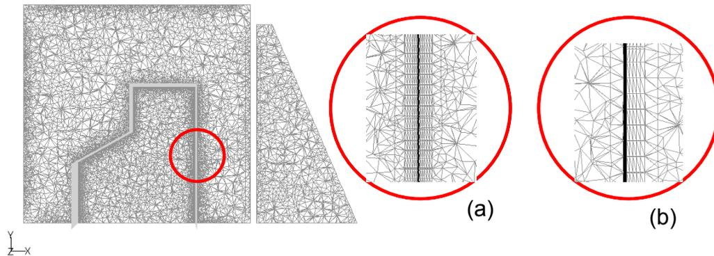
Figure 6 Grid in a cross section ( $z = 0$ ) (a) Mesh boundary layers on both sides of the object (b) Mesh boundary layers on the outside of the object
