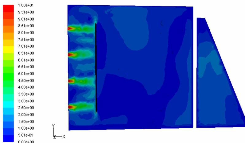
Figure 2 Velocity contours in a centre cross-section ( $z = 0$ )
