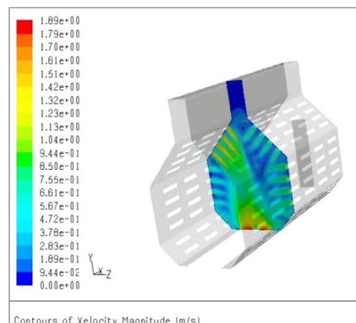
Figure 10 Velocity contours in a cross section in the empty chamber
