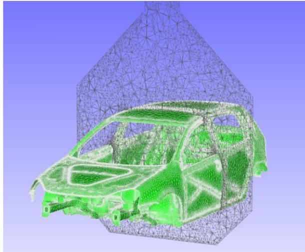
Figure 11 Mesh in a cross-section of the computational domain
