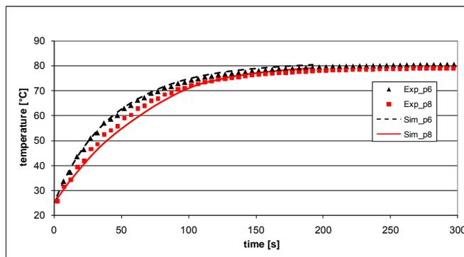
Figure 4 Comparison of heating-up curves on the KTL sheet
