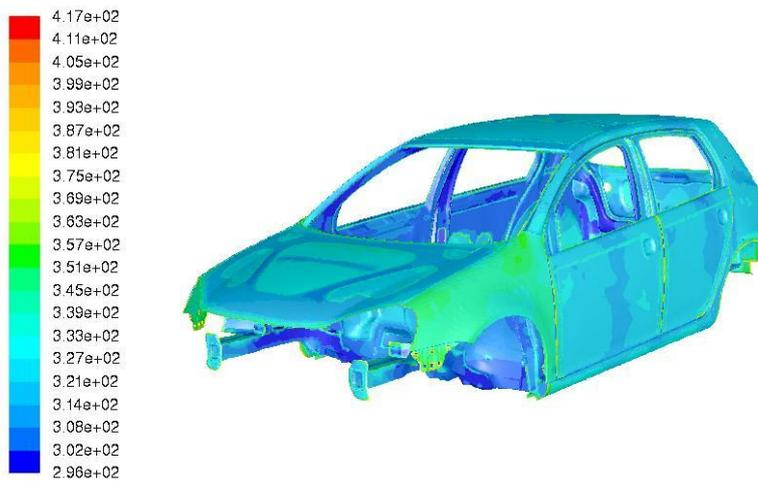
Figure 13 Temperature distribution (K) on car body surface at t = 20 s
