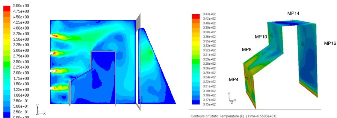
Figure 7: Simulation results in the Hygrex dryer (a) Velocity contours at  $z = 0$  (b) Temperature contours on the surface of the 3D model
