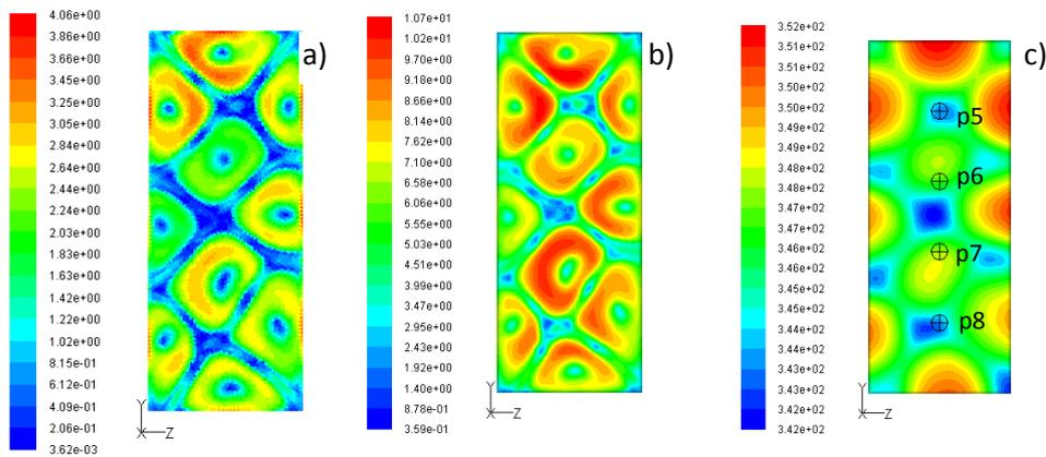
Figure 3 Contour distributions: a) Velocity contour (m/s) at wall-adjacent cells, b) non-dimensional wall distance  $y^+$  on the plate, c) temperature distribution (K) on the plate at  $t = 96$  s
