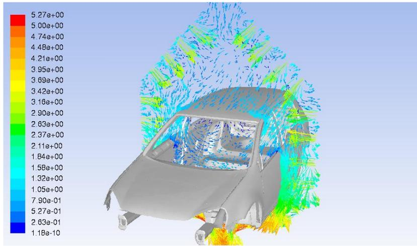
Figure 12 Velocity vectors (m/s) in a cross-section of the Eisenmann dryer
