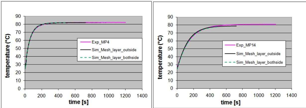
Figure 8 Comparison of heating-up curves on the surface of the 3D model
