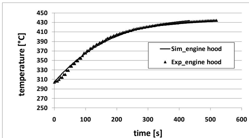
Figure 14 Comparison of heating-up curves on the car body
