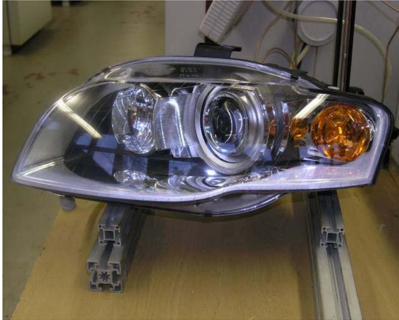
Figure 2: condensate on a prototype specifically designed for enhancing condensate formation
