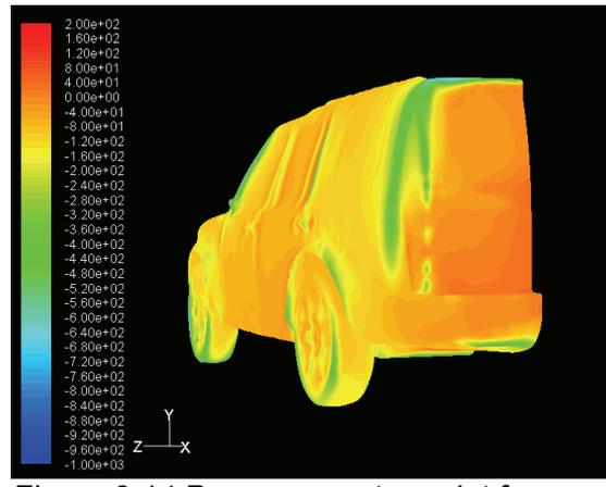
Figure 3.14 Pressure contour plot for config. 3 at 25m/s with 60° deflection
