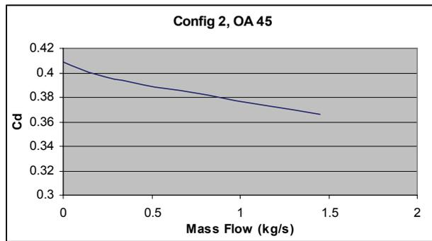
Figure 3.12 Drag values for config. 2 with flow angle of 45°
