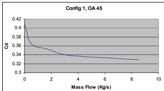
Figure 3.10 Drag values for config. 1 with flow angle of 45°
