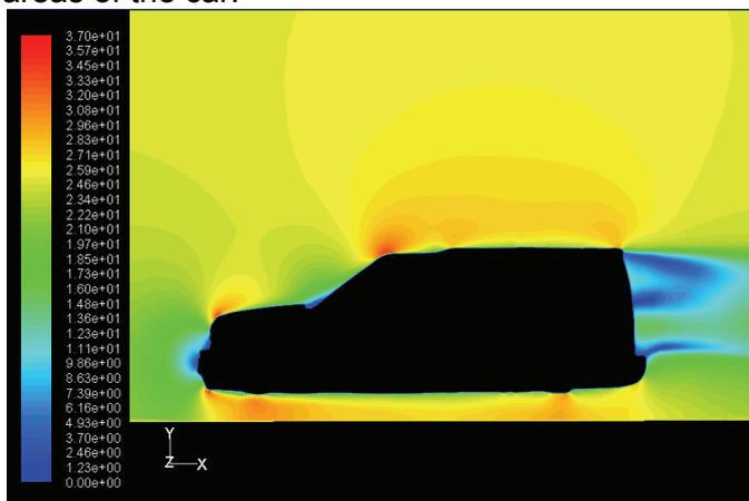
Figure 3.1 Velocity plot of airflow over standard model
