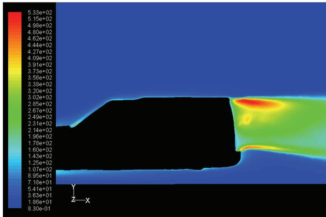
Figure 3.1 Turbulent intensity plot of standard model
